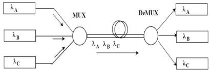
Fig 5.1 wavelenght division multiplexing
