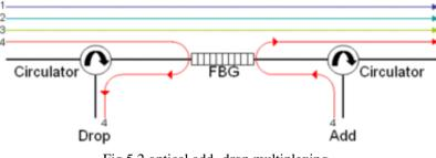
Fig.5.2 optical add- drop multiplexing
